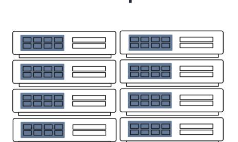
Lithium Iron Phosphate batteries store energy ready to be supplied when needed. These are stacked on top of each other to form a battery rack and are connected together to reach the required voltage and current of the BESS. These are a tried and tested technology that is commonly used in our day-to-day lives, such as in smartphones.
